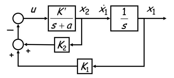
Given  $K_1$ , find the feedback gain,  $K_2$ , such that  $\int x_1^2 dt$  is minimal
