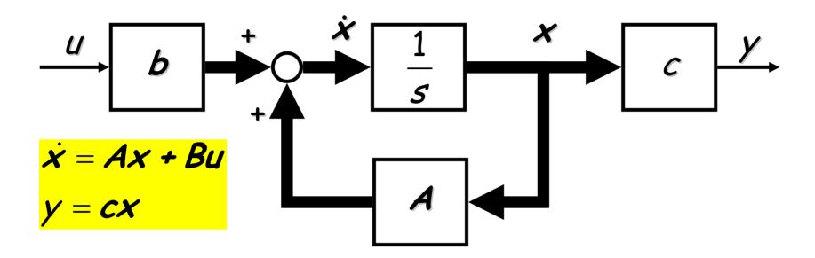
For SISO systems: u = input signal (scalar)y = output signal (scalar)  $b = \text{input matrix } (n \times 1)$  $x = \text{state vector} (n \times 1)$
