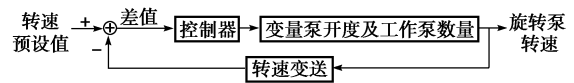
图3 旋转泵负反馈闭环控制方案 Fig.3 Scheme of negative feedback control for rotary pumps
