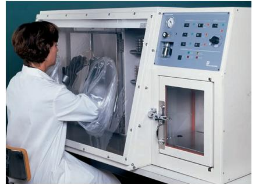
Figure 6.23 An Anaerobic Work Chamber and Incubator.
