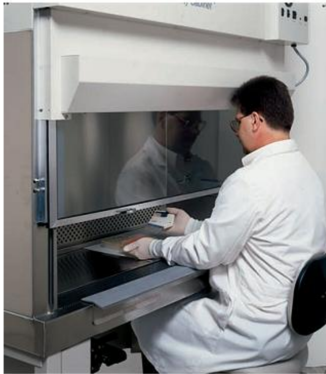
Figure 7.8 A Laminar Flow Biological Safety Cabinet. (a) A technician pipetting potentially hazardous material in a safety cabinet. (b) A schematic diagram showing the airflow pattern.
