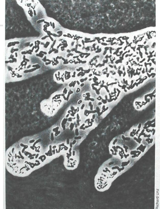
FIGURE 17.54 Photomicrograph of a floc formed by Zoogloea ramigera , the characteristic organism of the activated-sludge process. Note the large number of small, rod-shaped bacteria surrounded by a polysaccharide slime and the characteristic fingerlike projections of the floc. Negative stain using India ink.
